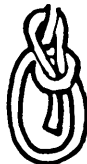
The bowline will not slip under strain, yet it is easily untied.
